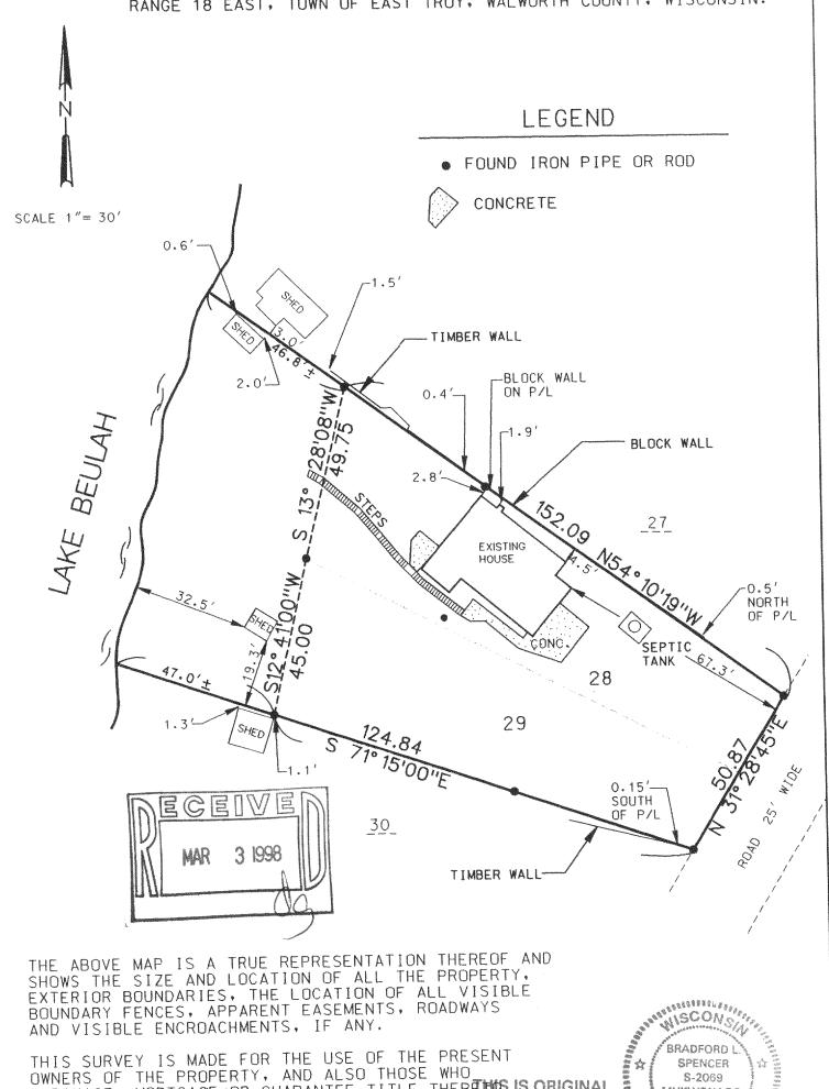
THE ABOVE MAP IS A TRUE REPRESENTATION THEREOF AND SHOWS THE SIZE AND LOCATION OF ALL THE PROPERTY, EXTERIOR BOUNDARIES, THE LOCATION OF ALL VISIBLE BOUNDARY FENCES, APPARENT EASEMENTS, ROADWAYS AND VISIBLE ENCROACHMENTS, IF ANY. THIS SURVEY IS MADE FOR THE USE OF THE PRESENT
